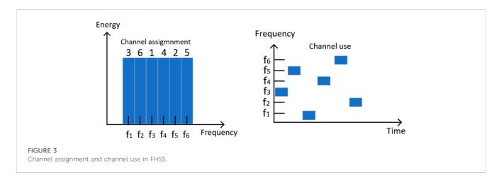
pseudo-random manner (Liu et al., 2017; Lei et al., 2018). For example, in a FHSS system, the transmitted signal is spread across multiple channels, as shown in Figure 3. The full bandwidth is divided into 6 channels, centred at  $f_1$  through  $f_6$ . The signal hops between them in the following sequence:  $f_3$ ,  $f_5$ ,  $f_1$ ,  $f_4$ ,  $f_6$  and  $f_2$ .
