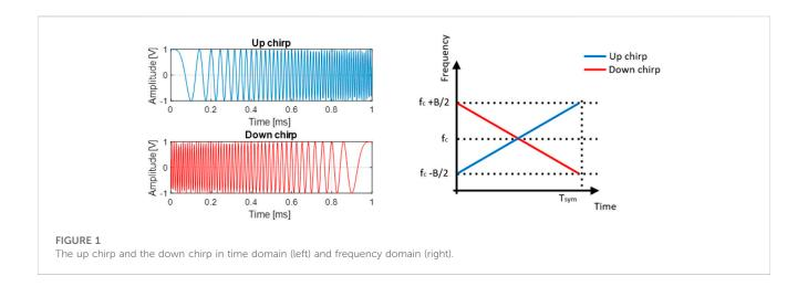
$$s(t) = \exp\left[j2\pi\left(f_c t + r t^2\right)\right], 0 \le t \le T_{sym} \tag{1}$$
