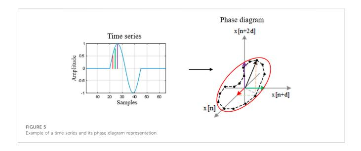
axis unit vectors and M = N - (m-1)d. As can be seen, two new parameters appear in the new representation vectors: the delay, which is usually determined with the mutual information method (Marwan et al., 2007) and the embedding dimension, which is usually determined with false nearest neighbor method (Webber and Zbilut, 1994). In Figure 5, you can see a graphic example that shows the transition from the time series to the phase diagram.
