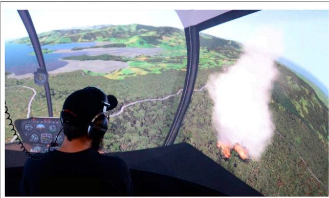
FIGURE 2 | CAVE system simulating helicopter cockpit for Air Attack Supervisor Training Clifford et al. (2018b).
