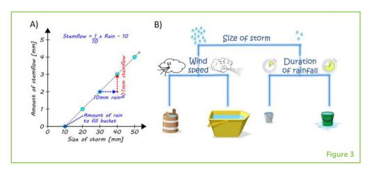
flowing. Once stemflow began, the tree canopy could drain 1 mm of every additional 10 mm of rain to the trunk as stemflow. So, we now have the bucket size (10 mm) and the stem drainage coefficient (1/10 = 10%) for this tree!
