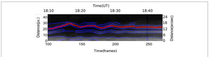
FIGURE 3 | Zoomed time-space diagram from Figure 2 with the Canny edge-detection output (blue lines) and the returned oscillation profile (red line) over-laid. The returned oscillation is qualitatively similar to the oscillation returned by Pascoe et al. (2016) for the same event.
