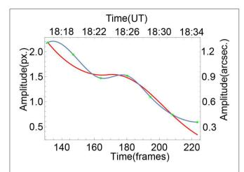
**FIGURE 7** | The dependence of the amplitude of the coronal loop oscillation on time. Green points correspond to maxima of the peaks plotted in **Figure 6**, the blue line is the fitted observed amplitude-time profile, and the red line represents the theoretical amplitude-time profile with  $\zeta=2.2$ ,  $\lambda=1.05$ ,  $\kappa=2.4$ , and  $\alpha=1.4$ .
