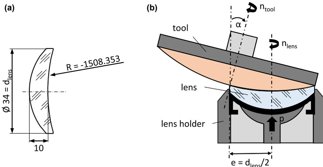
**Figure 5:** Boundary conditions for the application of the methodological approach. (a) Sketch of the lens to which the parameters are to be transferred. The drawing is not to scale. Only data approved by the manufacturer is shown. (b) Sketch of the process setup.
