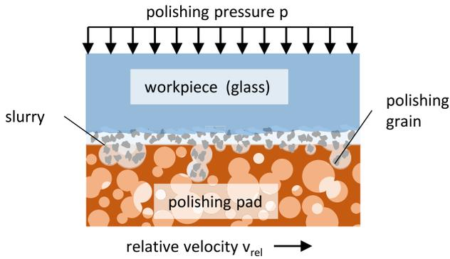
**Figure 1:** The effective system for the CMP of glass [1].
