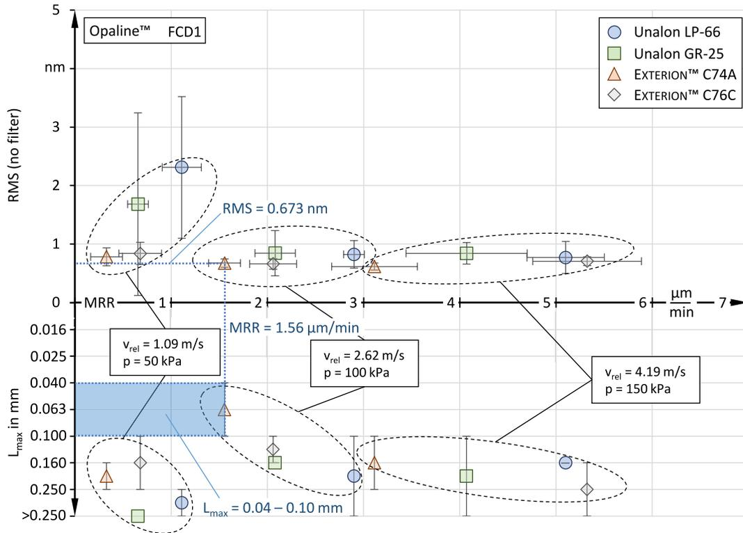
**Figure 3:** Illustration of the test results generated using the presented method and the components from Table 3. For a better overview, only selected parameter combinations are shown. The values of the three target variables MRR, RMS and  $L_{\max}$  are shown in the graph.
