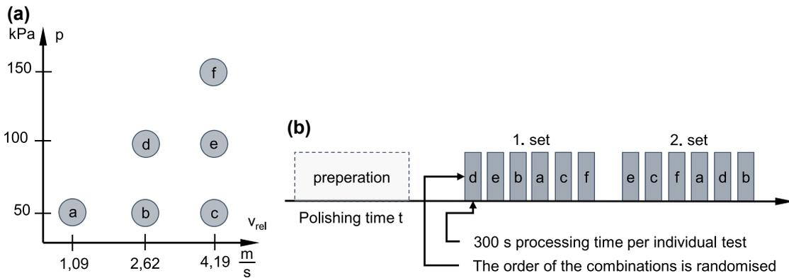
**Figure 2:** Design of the test procedure. (a) Combinations of polishing pressure and relative speed selected for implementation. (b) Sequence of individual tests. The order of the parameter combinations is randomised. Each specimen is polished for 300 s.
