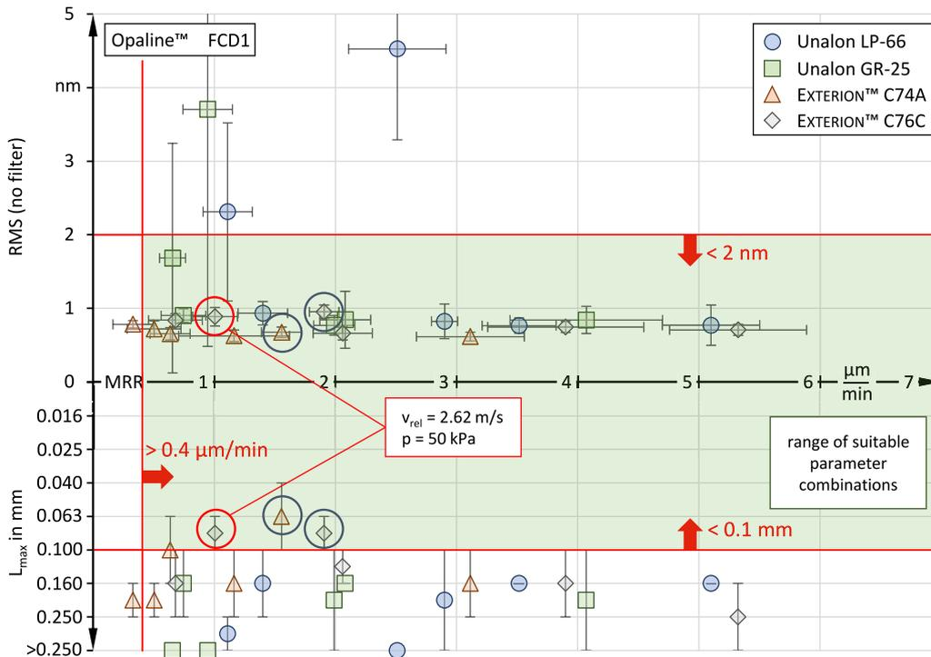
**Figure 4:** Illustration of the test results generated using the presented method and the components from Table 3. The boundary conditions for the target variables MRR, RMS and  $L_{max}$  are marked by red lines. The zone in which all requirements are met is highlighted in green. All suitable parameter combinations are highlighted. The selected set is additionally outlined in red.
