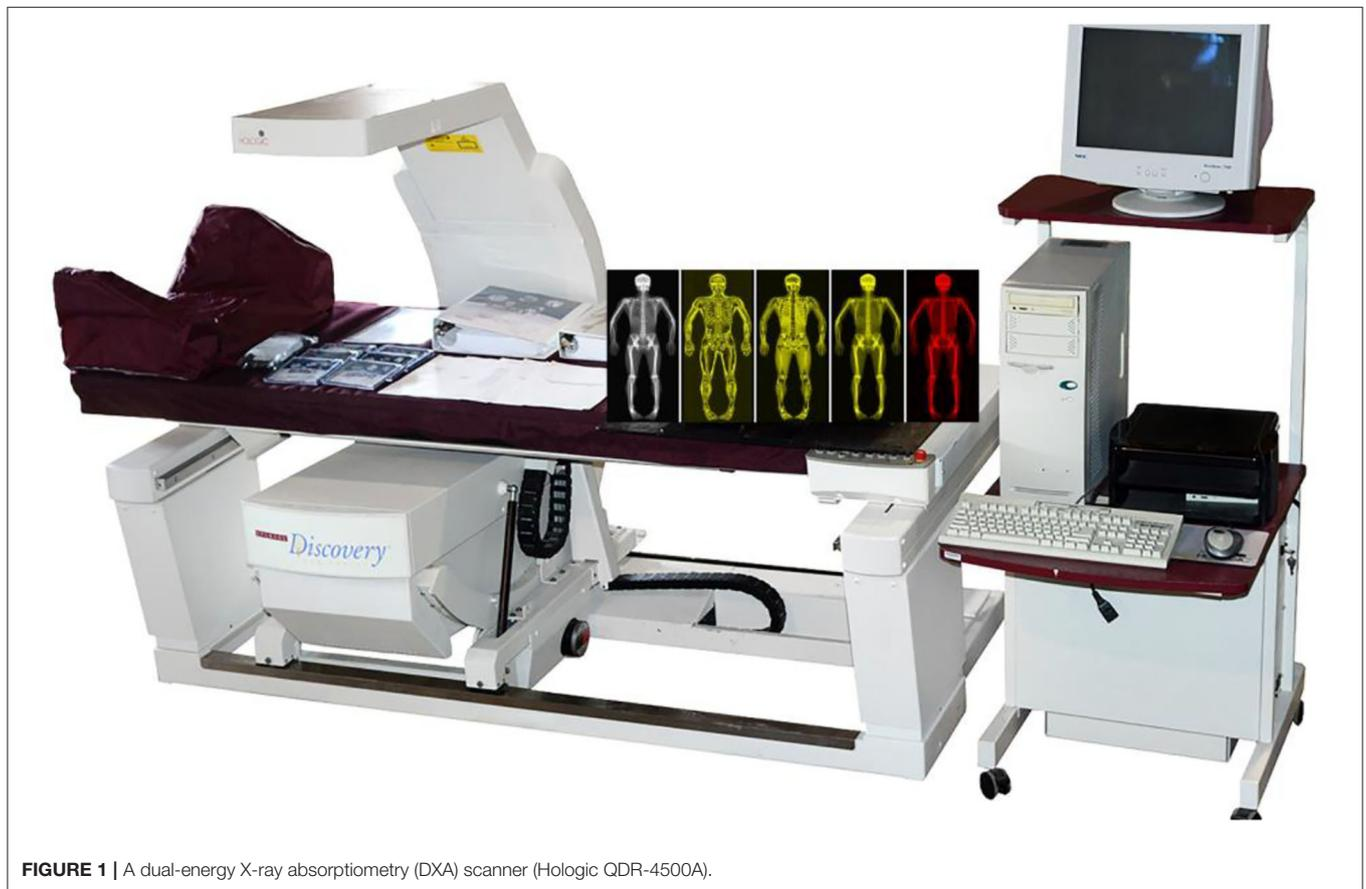
**FIGURE 1** | A dual-energy X-ray absorptiometry (DXA) scanner (Hologic QDR-4500A).
