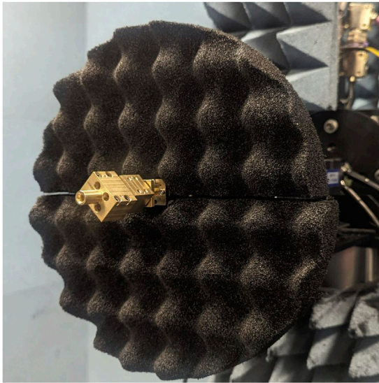
FIGURE 7 Measurement setup of the antenna. The polarizer is set to operate in the RHCP mode here.
