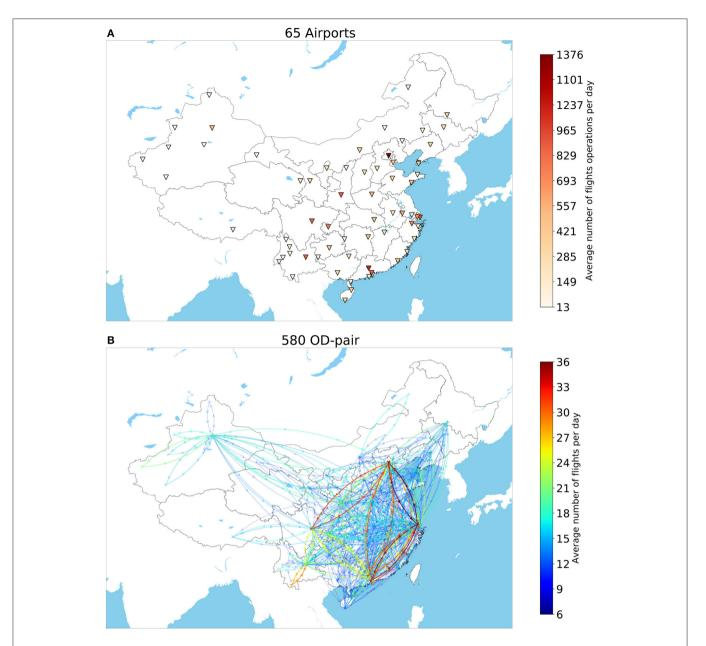
FIGURE 4 | The selected (A) 65 airports and (B) 580 OD-pair having more than 6 flights per day on average per Chinese aviation network in Quarter 3, 2017. Top: Airports are colored by the total number of flights operations per day including departures and arrivals; Bottom: OD pairs with clockwise directions are colored by the average number of flights operated per day.
