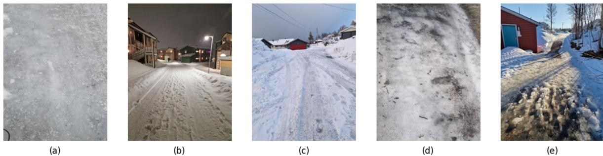
FIGURE 3 Various road conditions during data collection (a) road condition with black ice (b) road with fresh snow (c) road with crusted snow (d) road with gritted ice (e) road with wet slush.
