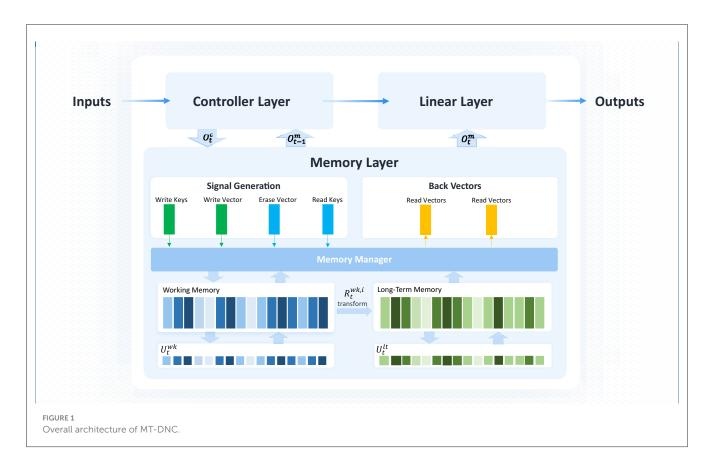
the MT-DNC model, which integrates two coordinated memory modules: working memory and long-term memory (Seo et al., 2016; Ba J. et al., 2016; Le et al., 2019, 2020). The proposed model improves both accuracy and convergence speed, offering superior performance compared to existing DNC-based models.
