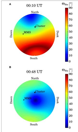
**FIGURE 12** |  $\Theta_{Bn}$  angle (between the IMF and the bow shock normal) at 00:10 UT **(A)** and 00:48 UT **(B)** in GSE. The Cluster and MMS positions projected on the bow shock are show with a star and a dot, respectively.  $\Theta_{Bn}$  of 45° (green) separate the quasi-parallel bow shock (blue) to the quasi-perpendicular bow shock (red/yellow).
