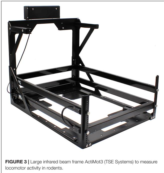
**FIGURE 3** | Large infrared beam frame ActiMot3 (TSE Systems) to measure locomotor activity in rodents.
