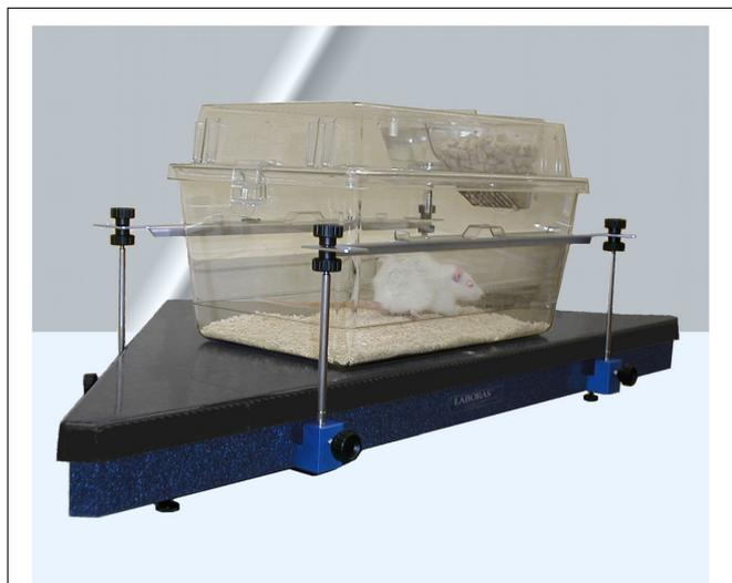
**FIGURE 4** | The measurement platform LABORAS turns animal's movement into electrical signals to analyze an extended set of rodent behavioral patterns (Metris b.v.).
