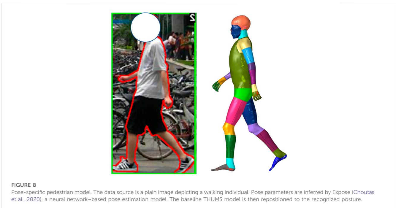
demonstrate three repositioned models. These models are ready for simulation, with comparable mesh quality as the baseline. The car-to-pedestrian simulation results suggest that diverse avoidance maneuvers lead to significantly varying impact responses.
