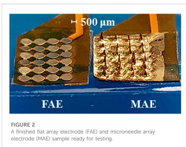
construction of microneedles, copper foils were firstly distributed on the substrate via the printed-circuit technique, and they all were electrically connected into one signal channel, forming a flat array electrode (FAE) (Figure 1A). The FAE was used as the inter-substrate for MAE fabrication and additionally used for performance comparison between MAE and FAE.
