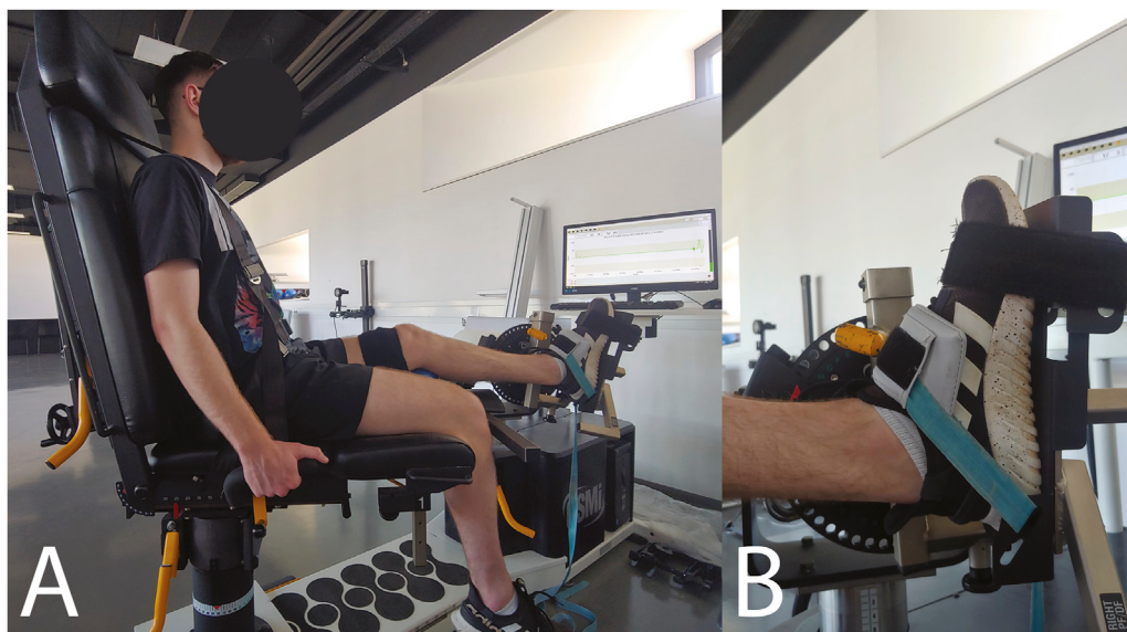
FIGURE 1 (A) Participant positioning and fixation in the dynamometer. (B) Close-up of ankle and foot fixation.
