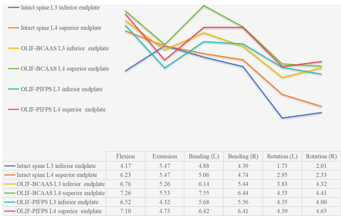
FIGURE 5 Line graph of the stress distribution on the L3 inferior and L4 superior endplates for the intact lumbar model and two OLIF surgical models under six motion modes.
