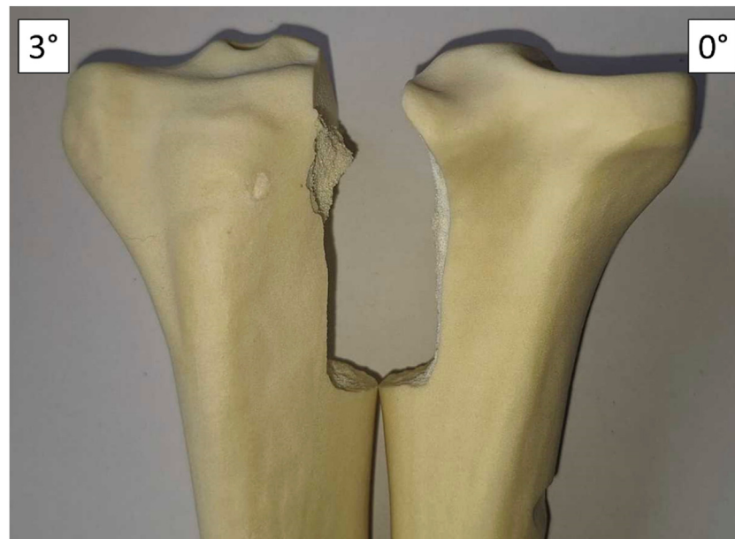
FIGURE 4 Fracture profiles of the tibiae with 3° and 0° varus inclination. At 3° inclination, the fracture becomes more complex and the fracture area is increased.
