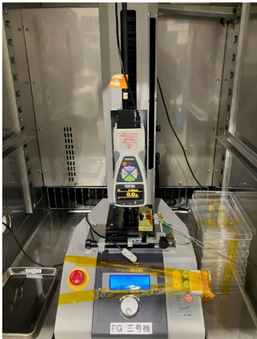
FIGURE 2 Load application test of the eR sensor using a force gauge installed within a constant temperature chamber. Capacitance was measured using an LCR meter placed externally.
