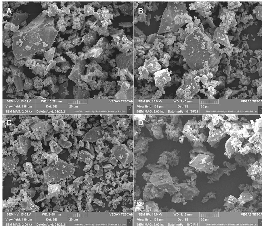
**FIGURE 2** | SEM images of the phosphate-based glass additives at  $\times 2,000$  magnification. Showing **(A)** P40 (custom-made) **(B)** P45 (custom-made) **(C)** P50 (custom-made), and **(D)** B65003 (commercial).
