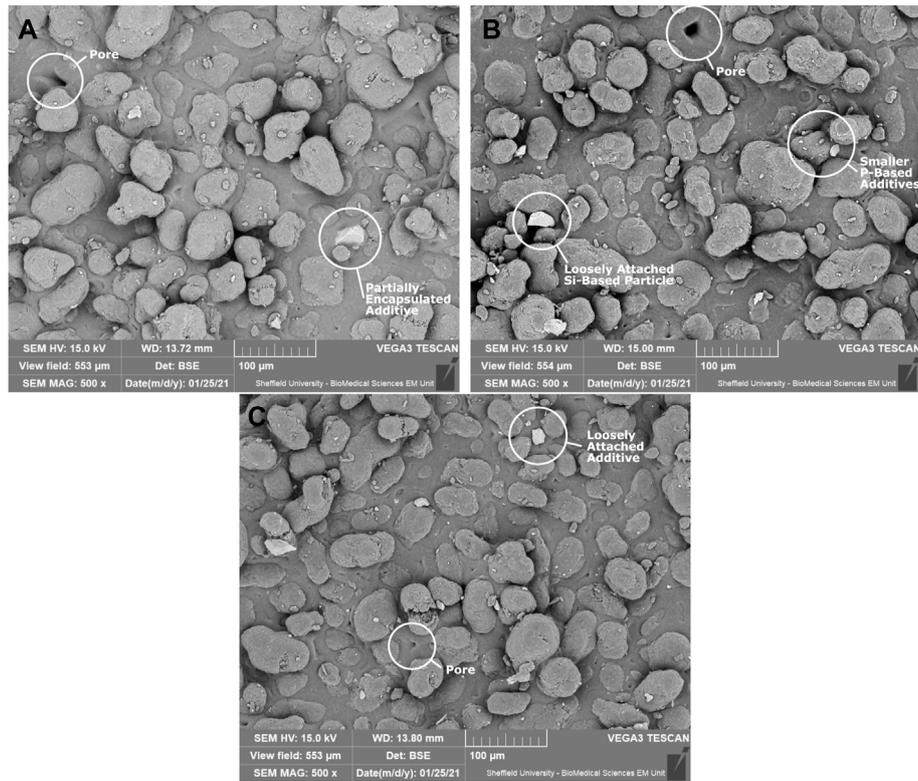
**FIGURE 6** | SEM images of the microcomposite surfaces containing the custom additives. The brighter features are additives, with the majority of the smaller features over the entire surface found to be the custom-made phosphorus-based additives. All features identified were found on all three materials. Shown are **(A)** 1% P40 Part **(B)** 1% P45 Part, and **(C)** 1% P50 Part.
