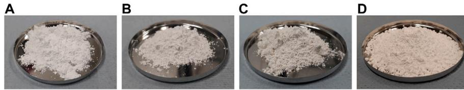
**FIGURE 1** | Photos of the three custom silver phosphate glass additives produced, each amount shown is approximately 20 g. Showing **(A)** P40, **(B)** P45, **(C)** P50, **(D)** commercial additive B65003.
