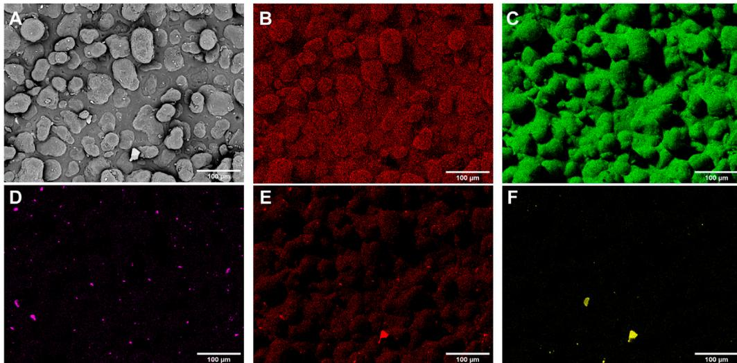
**FIGURE 7** | SEM and elemental maps on the surface of a 1% P50 microcomposite part obtained with EDX, with phosphorus indicative of the additive location. Shown are **(A)** SEM image **(B)** Gold **(C)** Carbon **(D)** Phosphorus **(E)** Oxygen, and **(F)** Silicon. Additional maps for Calcium, Magnesium and Titanium are not shown, with the concentration of silver too low to be detected.
