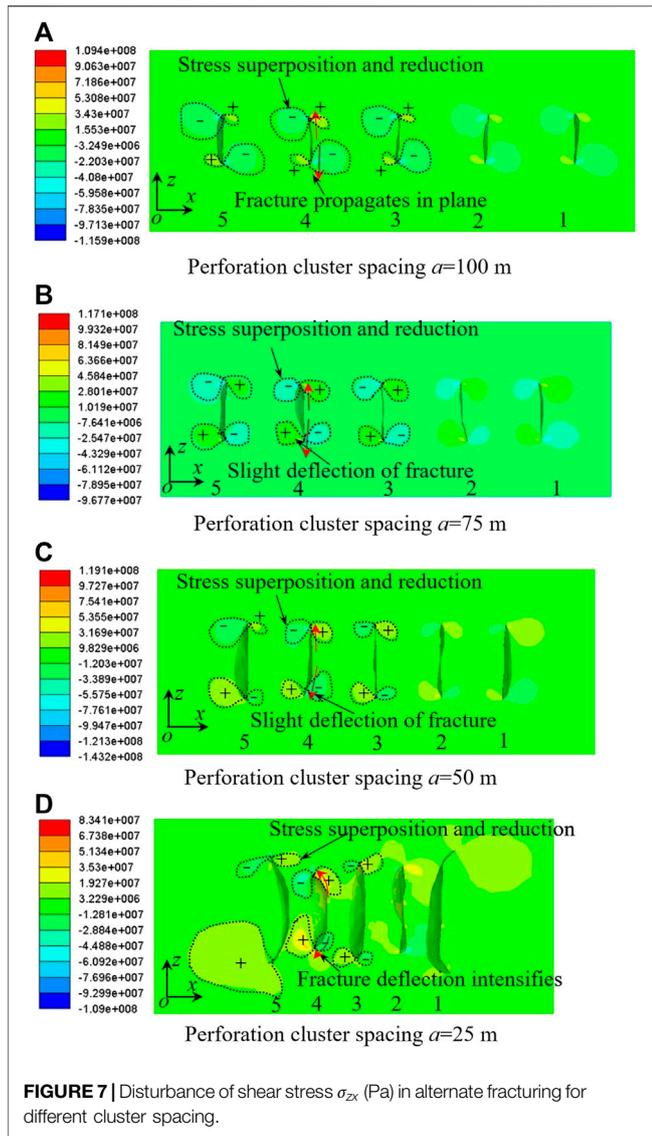
**FIGURE 7** | Disturbance of shear stress  $\sigma_{xz}$  (Pa) in alternate fracturing for different cluster spacing.
