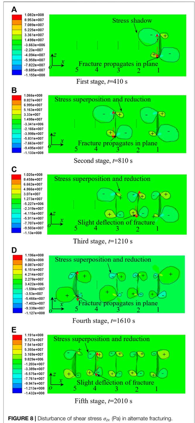
**FIGURE 8** | Disturbance of shear stress  $\sigma_{xz}$  (Pa) in alternate fracturing.
