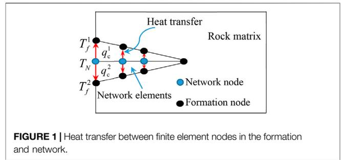
FIGURE 1 | Heat transfer between finite element nodes in the formation and network.
