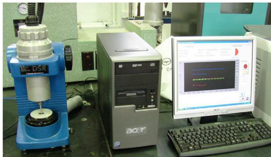
**FIGURE 1** | Dynamic shear rheometer (DSR) used in the study.
