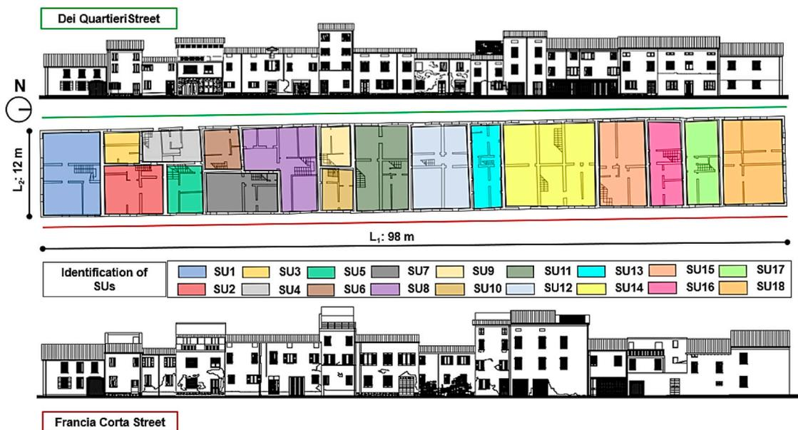
FIGURE 9 Division in SU of the masonry building compound in Mirandola (district of Modena, Italy).
