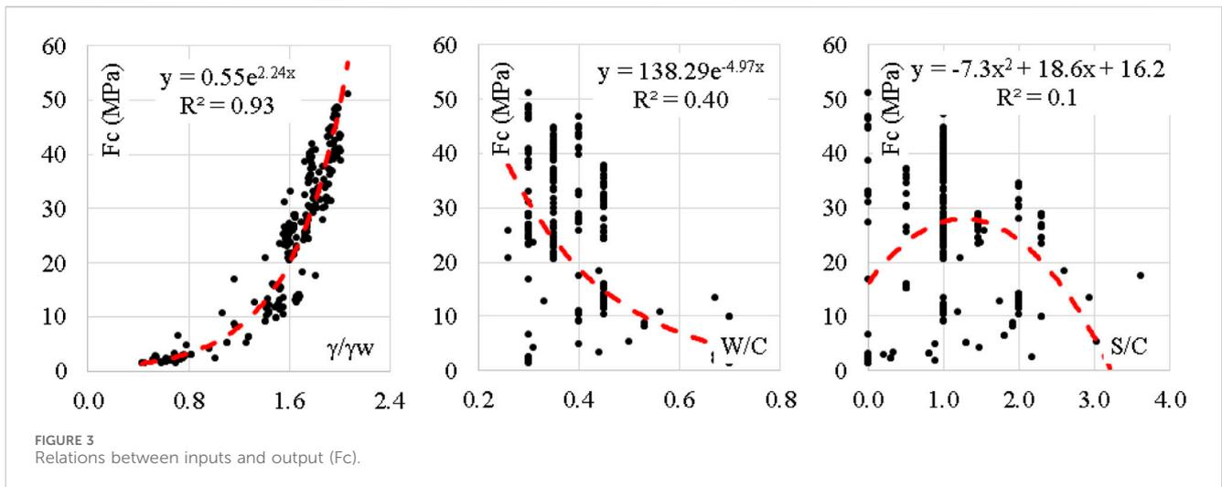
FIGURE 3 Relations between inputs and output (Fc).
