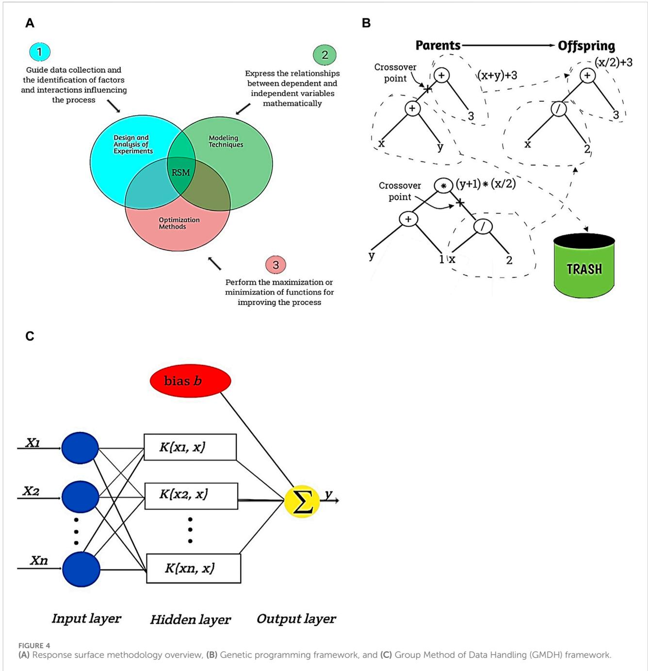
FIGURE 4 (A) Response surface methodology overview, (B) Genetic programming framework, and (C) Group Method of Data Handling (GMDH) framework.
