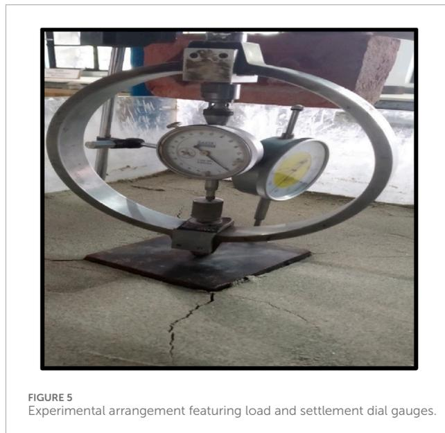
FIGURE 5 Experimental arrangement featuring load and settlement dial gauges.
