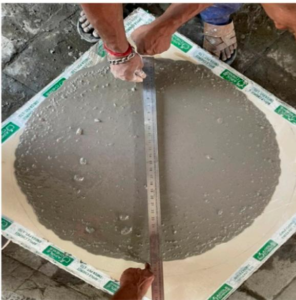
FIGURE 4 Slump flow.
