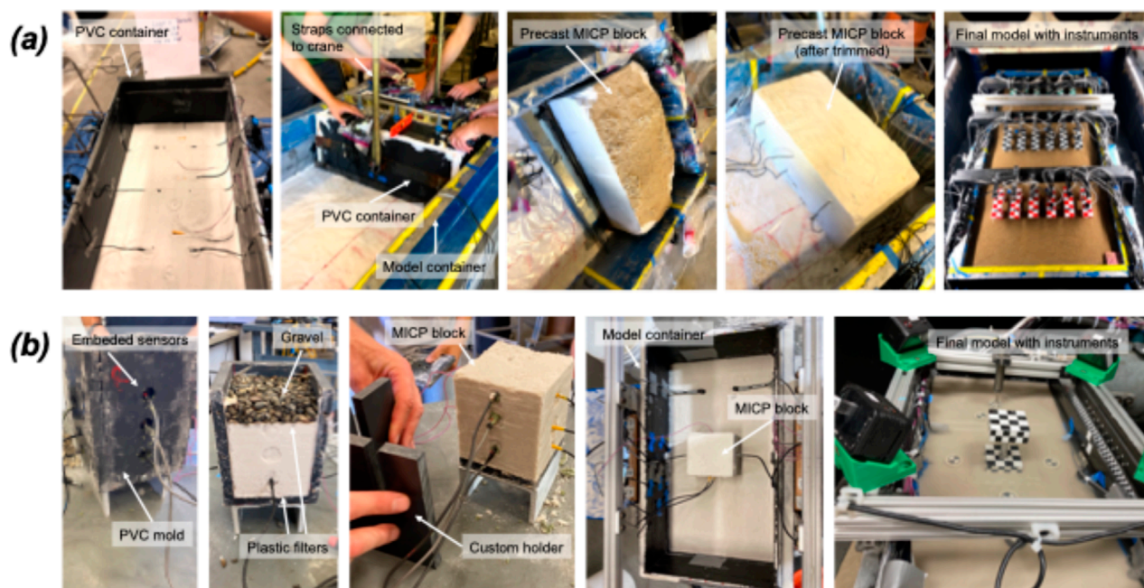
FIGURE 13 Model preparation process with discrete MICP-treated blocks: (a) 9-m centrifuge model and (b) 1-m centrifuge model.
