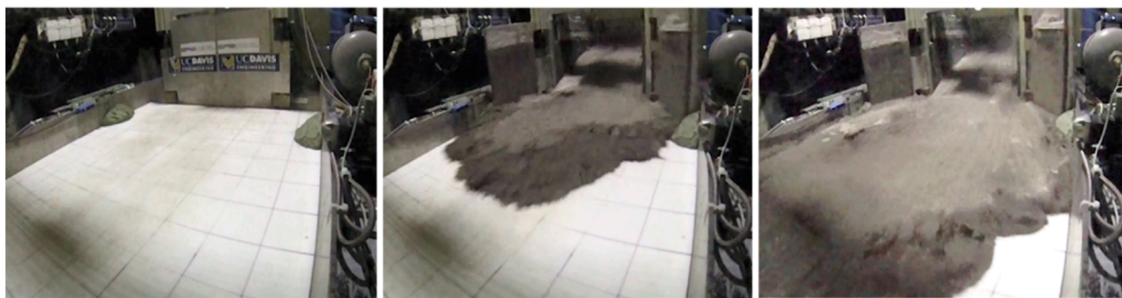
FIGURE 10 Sequence of failure of a saturated, loose deposit of coal ash tested at 60 g. The images were taken during a time period of about 1 s.
