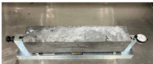
FIGURE 4 Measurement of total shrinkage, test rig and test specimen.
