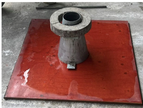
FIGURE 2 Slump flow at the RMC plant.
