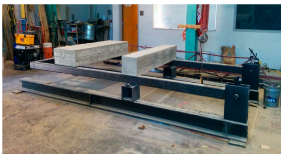
FIGURE 1 Experimental structure, initially proposed by Salyards and Noss (2014), modified and constructed at the University of South Carolina to evaluate structural responses in the 3–10 Hz frequency range.
