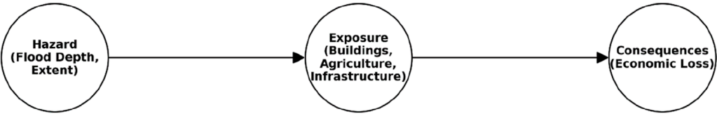
FIGURE 7 Schematic representation of the BN structure linking hazard, exposure, and consequence nodes.
