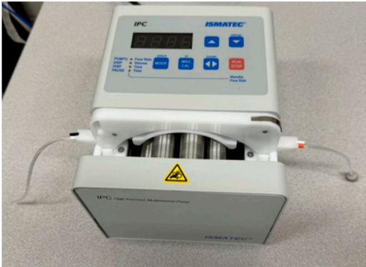
FIGURE 5 Installation of tubing with pump. Peristaltic pump with the cassette and Tygon tubing installed. Be sure to not crease the tubing.
