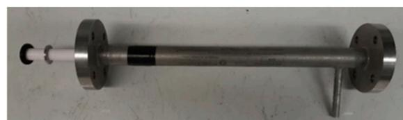
FIGURE 4 Test cell for monochannel tubular ceramic membranes.
