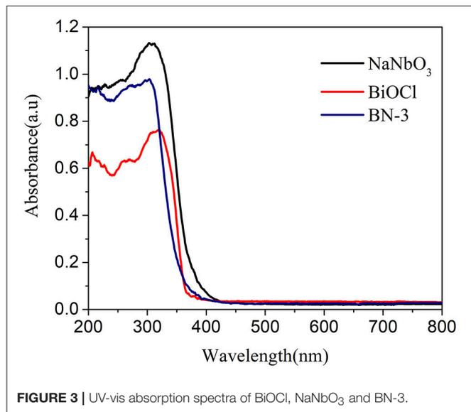
**FIGURE 3** | UV-vis absorption spectra of BiOCl, NaNbO<sub>3</sub> and BN-3.
