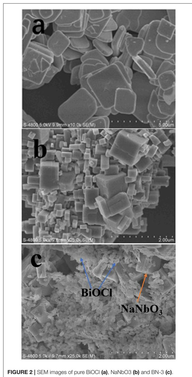
growth of BiOCl to larger ones. After analyzing the SEM image, the conclusion is in good agreement with the previous XRD analysis. BiOCl and NaNbO<sub>3</sub> form p-n junctions at the interface because of the close contact between BiOCl and NaNbO<sub>3</sub>. This improves the carrier transport rate and separation efficiency in photocatalysis and helps to improve the activity.
