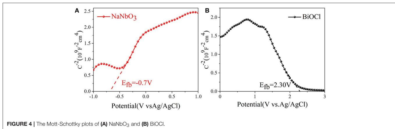
**FIGURE 4** | The Mott-Schottky plots of (A) NaNbO<sub>3</sub> and (B) BiOCl.
