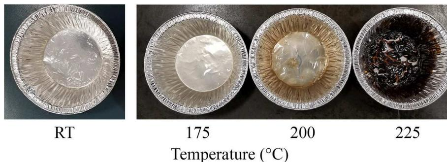
**FIGURE 3** | Image of CNC after oven drying colloid solution, which has been purified following acid hydrolysis of wood pulp that was hydrothermally treated at room temperature (RT) as control and 175–225°C appear brown with increasing intensity of the stain at 200 and 225°C.
