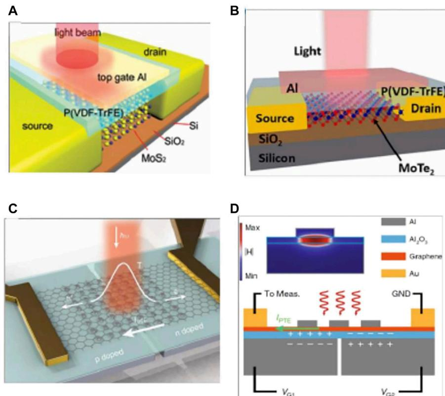
**FIGURE 9 | (A)** Photodetector based on ferroelectric polymer and MoS<sub>2</sub> (Wang et al., 2015b). **(B)** Photodetector based on ferroelectric polymer and MoTe<sub>2</sub> (Huang et al., 2016b). **(C)** Plasmonic microcavity integrated graphene photodetector (Wang et al., 2020). **(D)** Cross-sectional schematic of the graphene photodetector with split gates and a nano disk (Wang et al., 2020).
