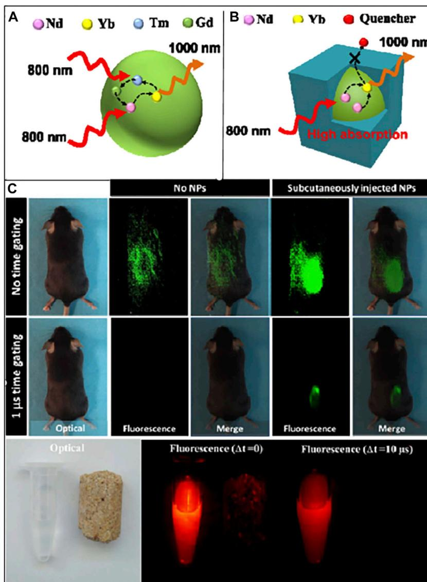
**FIGURE 6 | (A)** Schematic diagram of energy transfer in NaYF<sub>4</sub>:Yb<sup>3+</sup>, Nb<sup>3+</sup>, and Tm<sup>3+</sup>NPs, **(B)** the core/shell structure of NaYF<sub>4</sub>:Yb<sup>3+</sup>, Nb<sup>3+</sup>@CaF<sub>2</sub>NPs, **(C)** optical and NIR images of C57BL/6 mice and NaYF<sub>4</sub>:Yb<sup>3+</sup>, Nb<sup>3+</sup>@CaF<sub>2</sub> (George et al., 2013).
