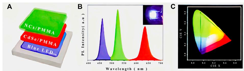
**FIGURE 5 | (A)** Schematic illustration of the configuration, **(B)** PL spectra (Inset shows a photograph of the device) and **(C)** CIE color coordinate of the CsPbBr<sub>3</sub>/SiO<sub>2</sub> based WLED (Li et al., 2015).
