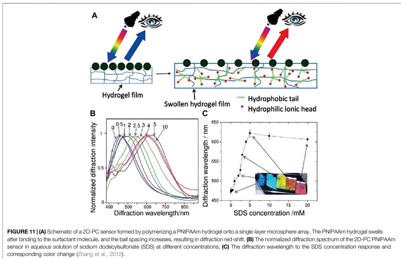
in the microcavity is combined with the biotin bovine serum albumin molecule (b-BSA), the resonance wavelength in the microcavity changes, and when the concentration of b-BSA changes, the concentration can be detected by measuring the standard curve of the change in the wavelength position of the resonance peak. Zhang et al. (2012) developed a two-dimensional photonic crystal sensing material for visual detection of anionic
