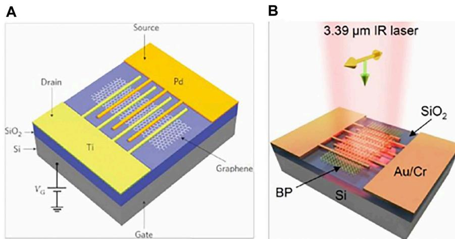
**FIGURE 8 | (A)** MGM photodetector with heterogeneous metal interdigital electrode (Mueller et al., 2010); **(B)** BP mid infrared detector integrated interdigital electrode (Guo et al., 2016). (Neto et al., 2007)
