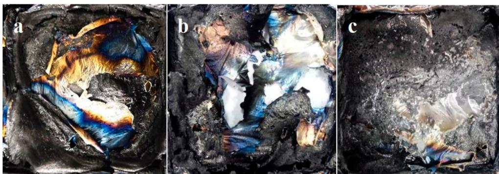
**FIGURE 9** Photograph of the residual carbon layer of the PLA/P-PPD-Ph/ECE flame retardant composite after conical calorimetry: (A) PLA/P-PPD-Ph/ECE-0%, (B) PLA/P-PPD-Ph/ECE-4%, (C) PLA/P-PPD-Ph/ECE-8%.
