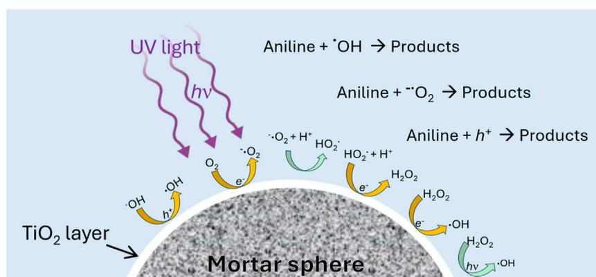
FIGURE 6 Schematic illustration for photocatalysis mechanism of TiO<sub>2</sub> immobilized on the substrate.
