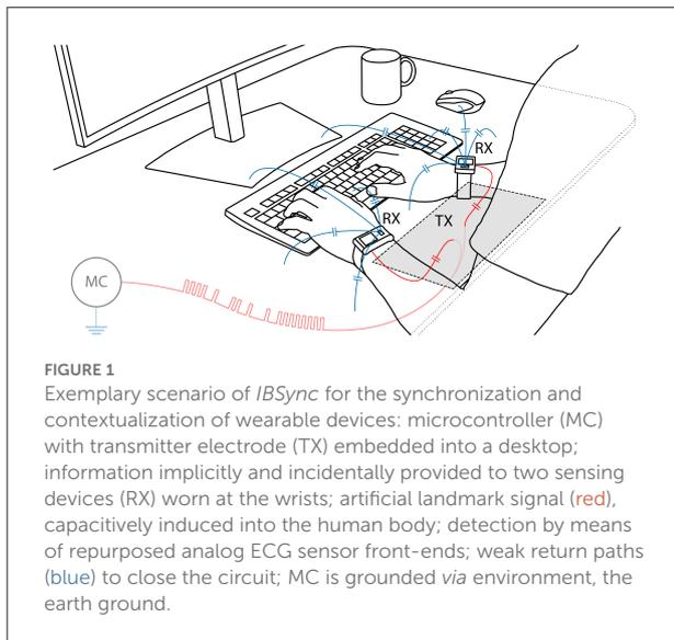
microcontroller<sup>2</sup> from Texas Instruments directly drives the signal electrode and hence modulates its surrounding quasi-static electric field. Unlike for antennas in radio frequency (RF), there are no special requirements on the electrode since rather low frequencies are applied. It is made from metal foil and has a relatively large size of  $16 \times 32 \text{ cm}^2$  to provide a sufficiently wide contact face.
