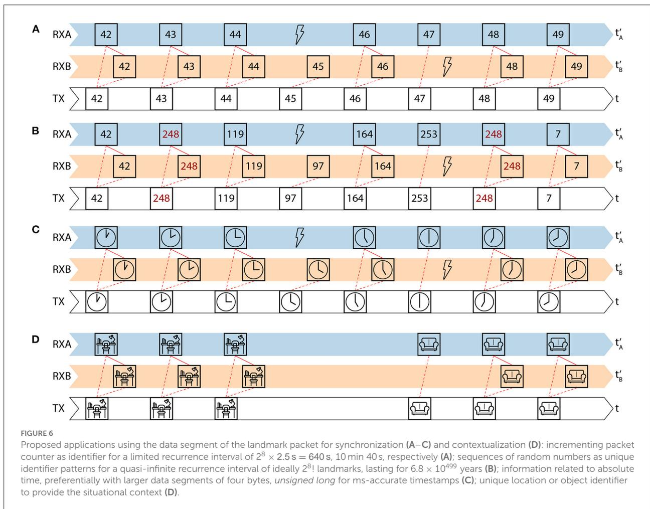
scheme (Figure 6C). A longer data segment of two, three, or even four bytes for an *unsigned long* ms-accurate timestamp would significantly upgrade this concept, however at cost of robustness against disruption through motion.
