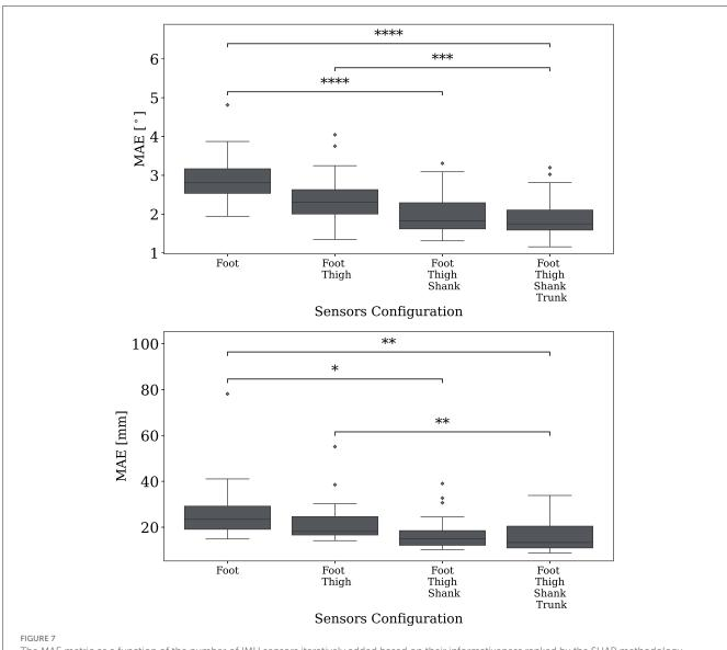
The MAE metric as a function of the number of IMU sensors iteratively added based on their informativeness ranked by the SHAP methodology across the four body sectors, with the upper plot showing slope prediction case and the lower plot showing stair height prediction case. Statistical significance is denoted by asterisks, with  $*p \le 0.05$ ,  $*p \le 0.01$  \*\* $*p \le 0.001$ \*, and  $*p \le 0.001$ \*.
