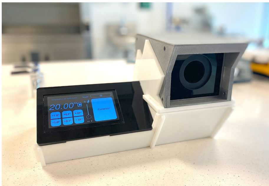
FIGURE 6 Laboratory calibrator for infrared tympanic thermometers (ITTs) in operation. (Front view of the device showing the touch display and the cavity).
