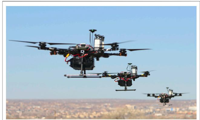
**FIGURE 1** | Flocking Dragonfly UAVs in formation. The flocking Dragonfly UAVs are used to survey volcanic CO<sub>2</sub> plumes.
