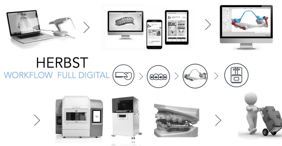
FIGURE 7 Full-digital workflow of the appliance production.
