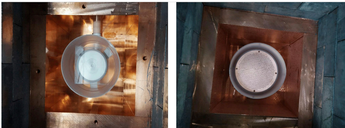
FIGURE 2 Bare PMMA plate (left) and FAT-GEM (right) inside the copper shielding of the setups used for radioactivity screening at Laboratorio Subterráneo de Canfranc.
