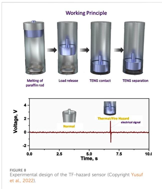
temperature of 60°C–70°C was reached (80°C for the metallic case), the message of FIRE DANGER could be visualized in the TTS platform on any electronic device with access to the internet. Third, an Arduino SIM808 GPS/GRPS/GSM shield connected to an Arduino board was programmed in such a way that as soon as the V peak generated by the TENG was detected, an SMS with the message of FIRE DANGER (or other) would be sent to a smart phone. The photo of the TF-hazard sensor is shown in Figure 8.
