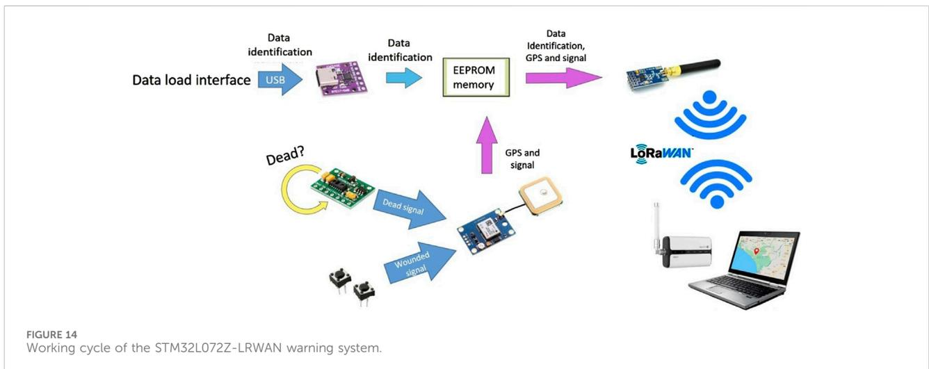
FIGURE 14 Working cycle of the STM32L072Z-LRWAN warning system.
