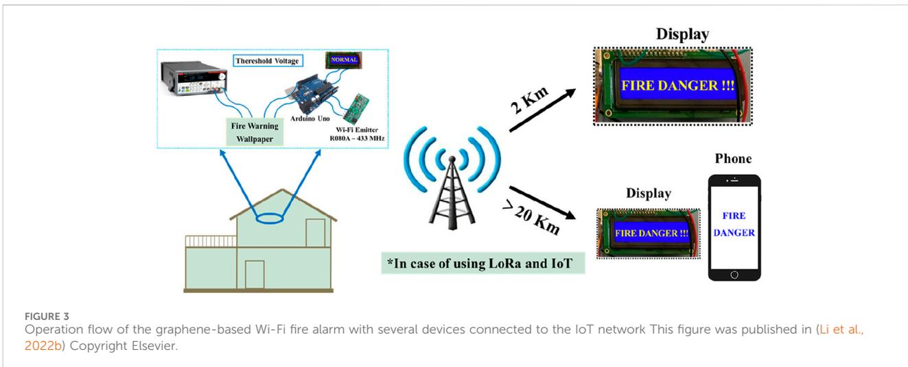
FIGURE 3 Operation flow of the graphene-based Wi-Fi fire alarm with several devices connected to the IoT network This figure was published in (Li et al., 2022b) Copyright Elsevier.
