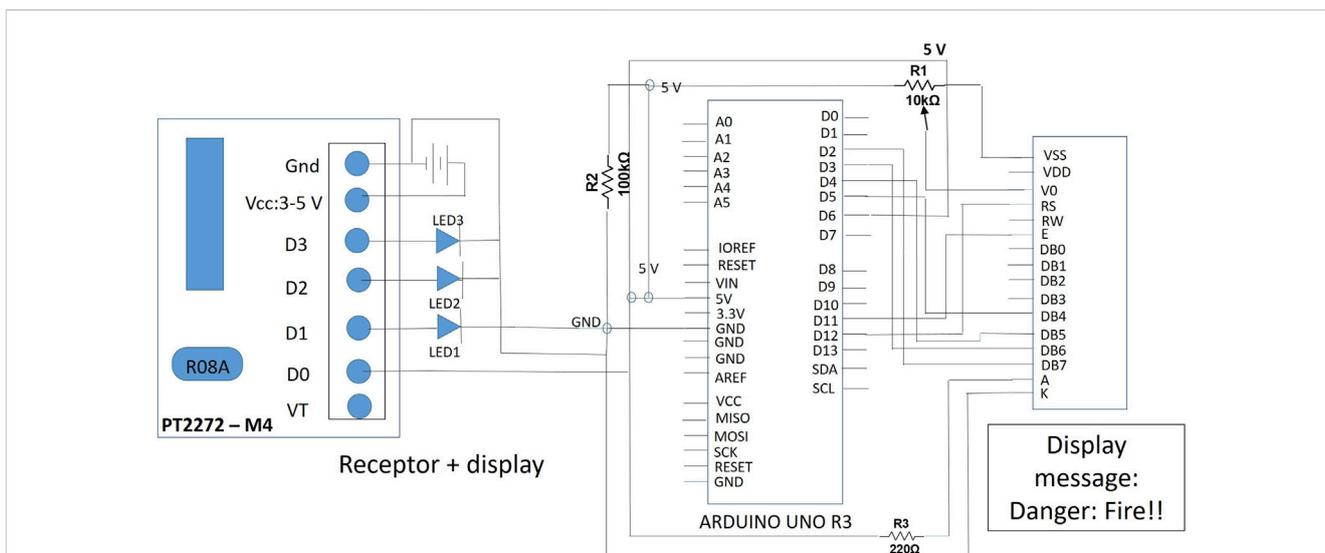
**FIGURE 2** Schematics of the warning fire alarm part corresponding to the Wi-Fi receptor unit and the Arduino connected to three LEDs and to an LCD. This receptor unit was programmed with the Liquid Crystal library with the aim of showing a typical alarm message. This figure was published in (Li et al., 2022b) Copyright Elsevier.
