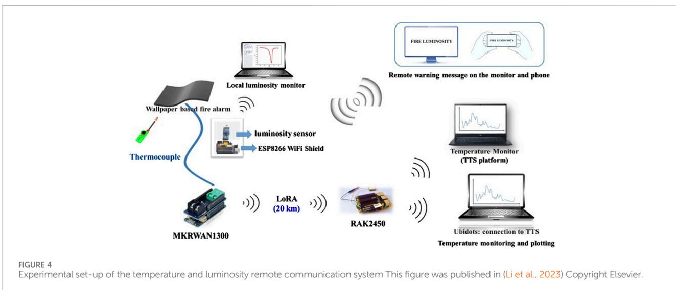
FIGURE 4 Experimental set-up of the temperature and luminosity remote communication system This figure was published in (Li et al., 2023) Copyright Elsevier.
