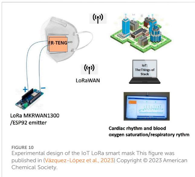
Different V-signals generated by the TENGs were monitored in Ubidots using the TTS platform (Vázquez-López et al., 2023). Examples of excited and relaxed states of a patient’s breathing could be observed *in situ* by using the LoRa protocol in a smart screen connected to the Internet (see Figure 11).
