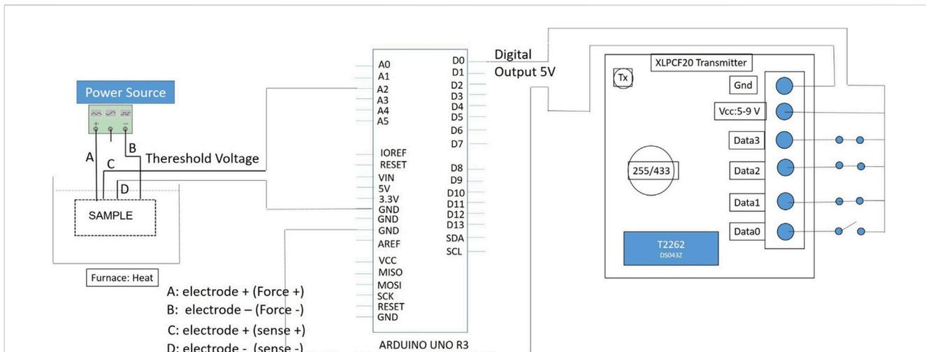
**FIGURE 1** Schematics of the warning fire alarm part corresponding to the following: the power source connected to a paper by two force electrodes, the sensing electrodes connected to the Arduino that works as an ADC with a characteristic threshold, and the XLPCF20 Wi-Fi transmitter that will send the Wi-Fi signal to the R08A receptor. This figure was published in (Li et al., 2022b) Copyright Elsevier.
