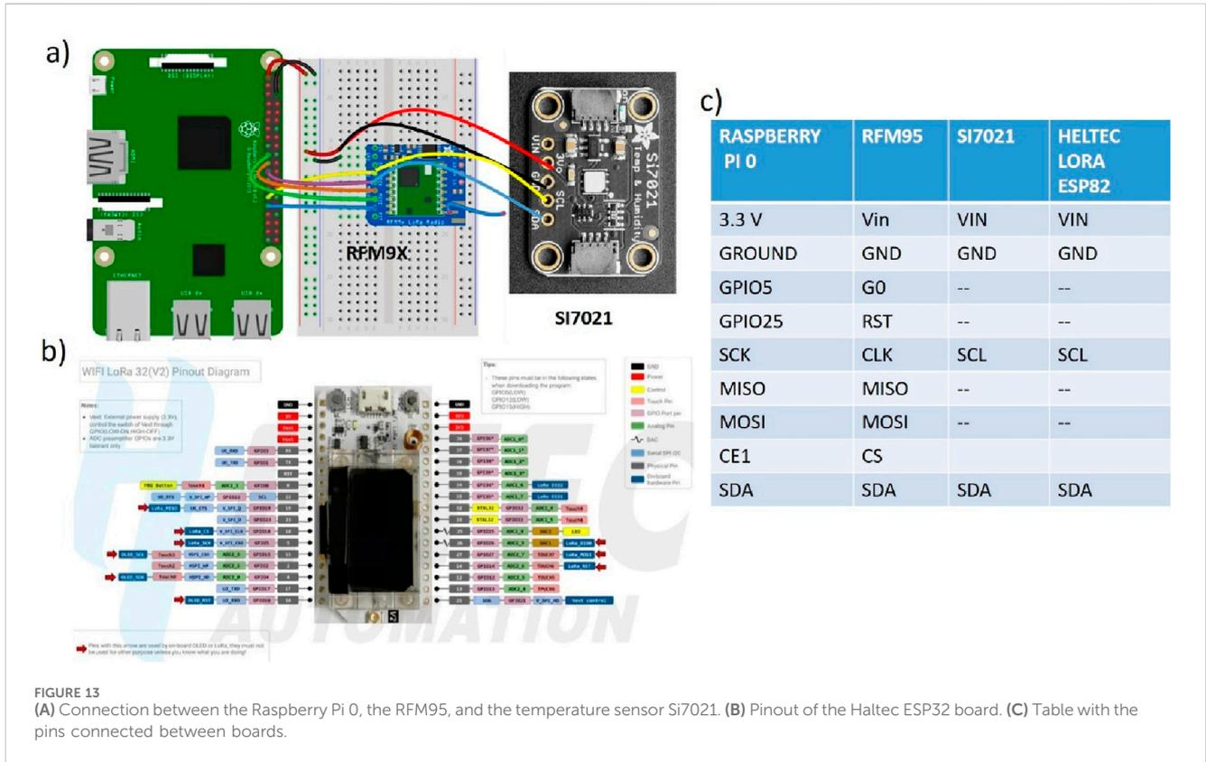
FIGURE 13 (A) Connection between the Raspberry Pi 0, the RFM95, and the temperature sensor Si7021. (B) Pinout of the Haltec ESP32 board. (C) Table with the pins connected between boards.
