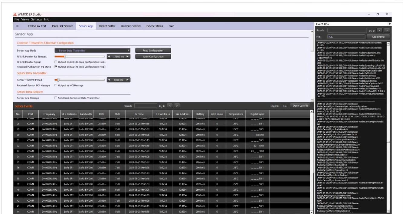
FIGURE 18 WiMOD LR interface, where communication (temperature values) between LoRa modules is shown.
