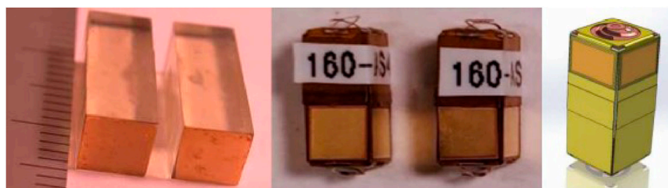
FIGURE 6 TlBr crystals with electrodes, and packaged VFG TlBr detectors with 3D drawing model. The TlBr ingots were grown by RMD using the zone melting technique. The bars were cut, polished, and etched in a bromine-methanol solution. The longest dimension of the device aligns with, or is parallel to, the growth direction. Platinum contacts were sputtered on the cathode and anode sides.
