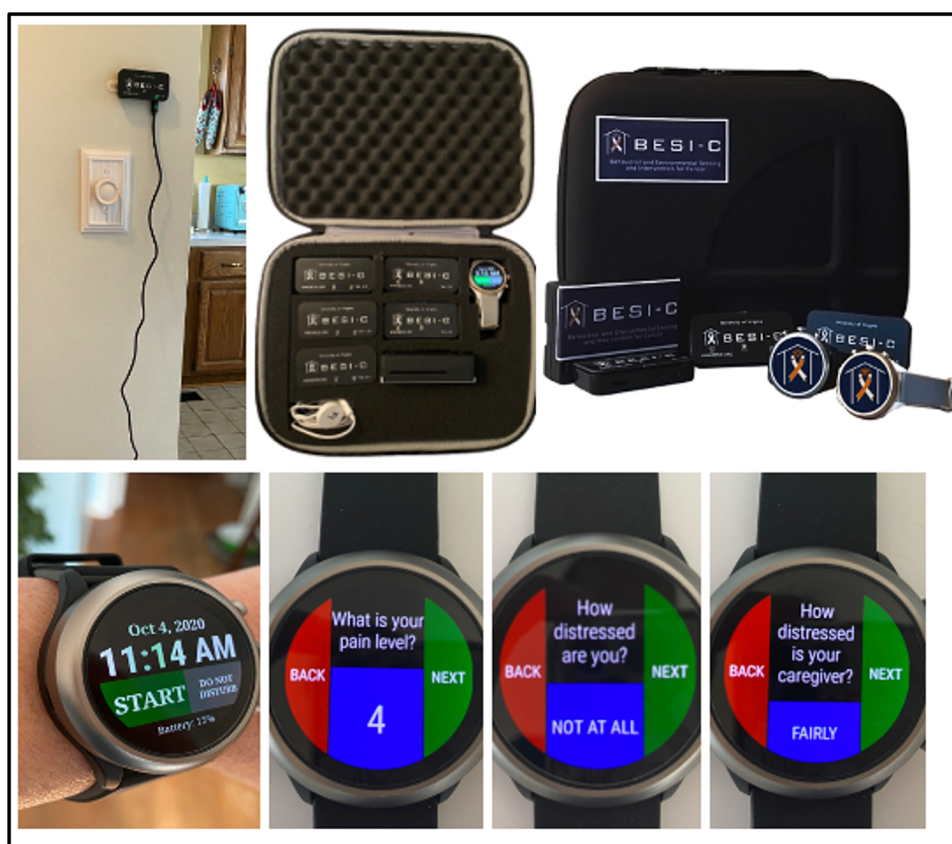
FIGURE 1 BESI-C system components: Top, environmental sensor and “BESI Box”; bottom, BESI-C custom wearable application and examples of ecological momentary assessments (EMAs).
