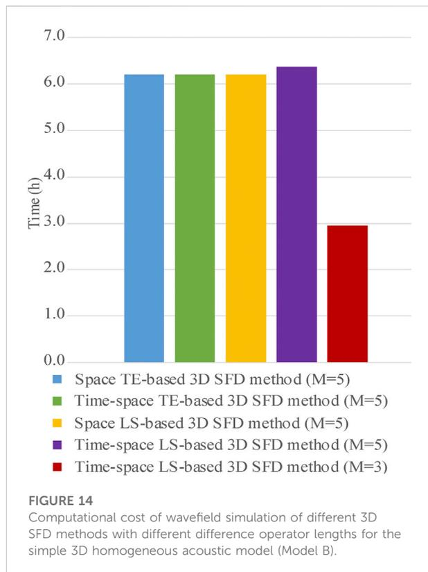
computational cost analysis, we should estimate and store the difference coefficients of our optimized time-space domain LS-based 3D SFD method in advance before wavefield modeling to effectively reduce the computing time of whole forward modeling for a given 3D model. This strategy can effectively reduce the difficulty of applying our optimized time-space domain LS-based 3D SFD method to 3D RTM, because it does not cause too much unnecessary time consumption during wavefield extrapolation.
