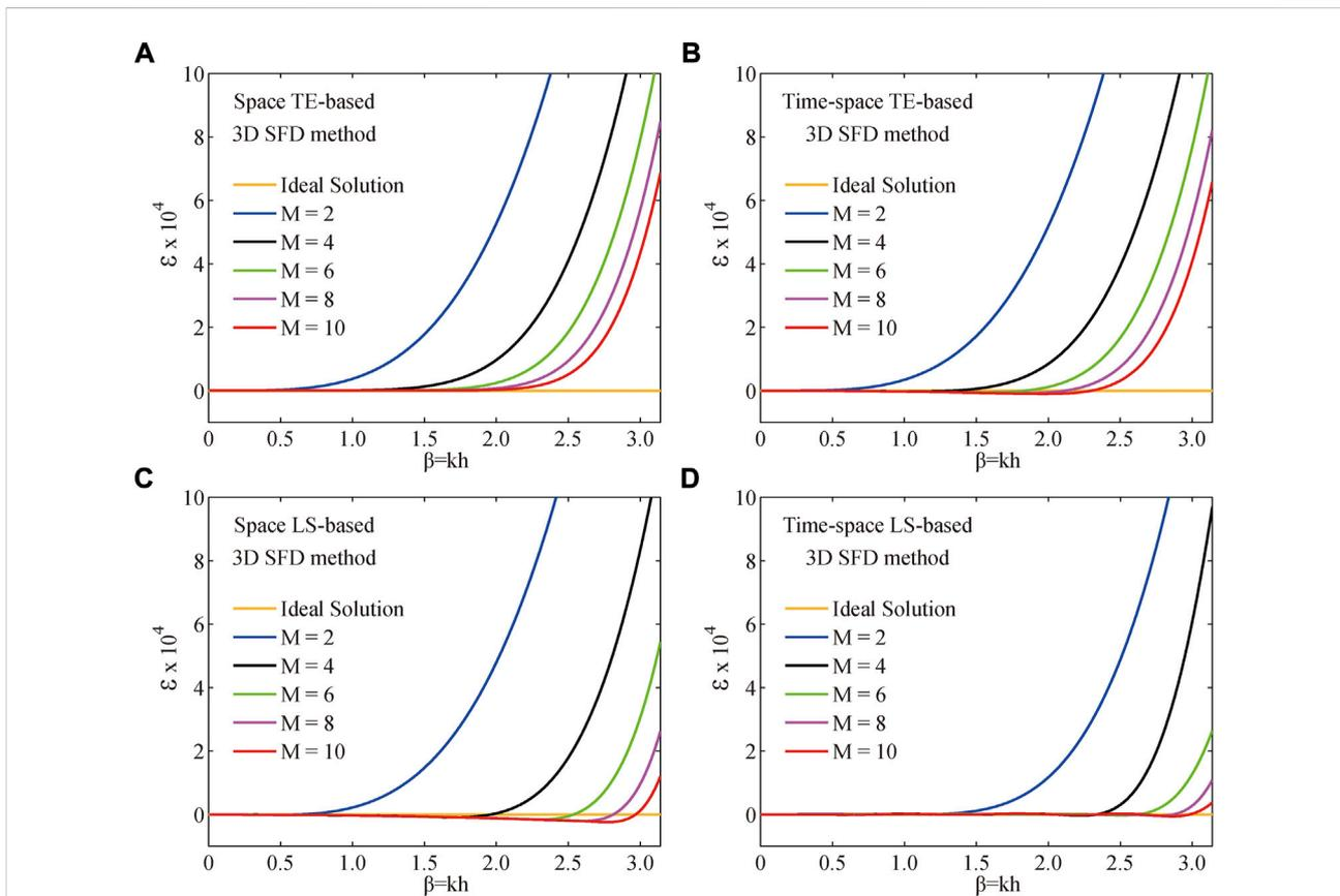
**FIGURE 1** Variation curves of numerical dispersion ( $\epsilon$ ) with the difference operator length ( $M$ ) changing for the simple 3D homogeneous acoustic model (Model A). These subgraphs (A–D) indicate different 3D SFD methods listed in themselves.
