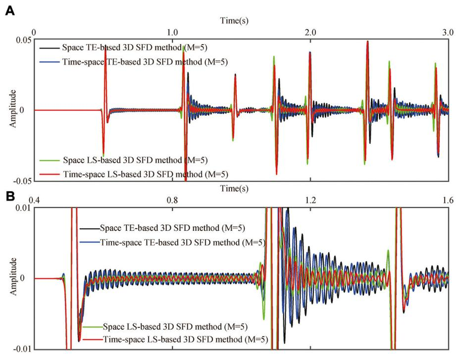
**FIGURE 8** Vibration curves simulated by different 3D SFD methods ( $M = 5$ ) for the simple 3D homogeneous acoustic model (Model B) at particle  $(x, y, z) = (1.0 \text{ km}, 1.0 \text{ km}, 2.0 \text{ km})$ . **(A)** Full vibration curves. **(B)** Local magnification curves.
