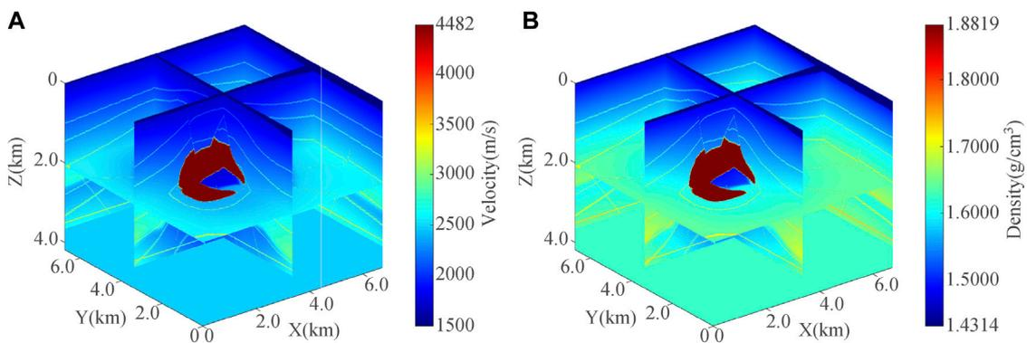
**FIGURE 9** 3D SEG/EAGE salt model. **(A)** Velocity. **(B)** Density.
