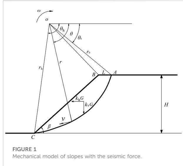
FIGURE 1 Mechanical model of slopes with the seismic force.
