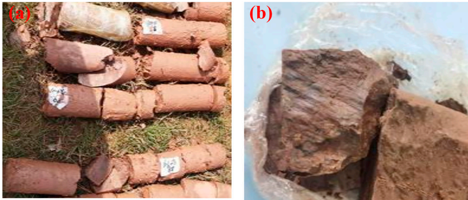
FIGURE 2 Schematic diagram of mudstone joints and fissures. (A) Mudstone core. (B) Massive mudstone.
