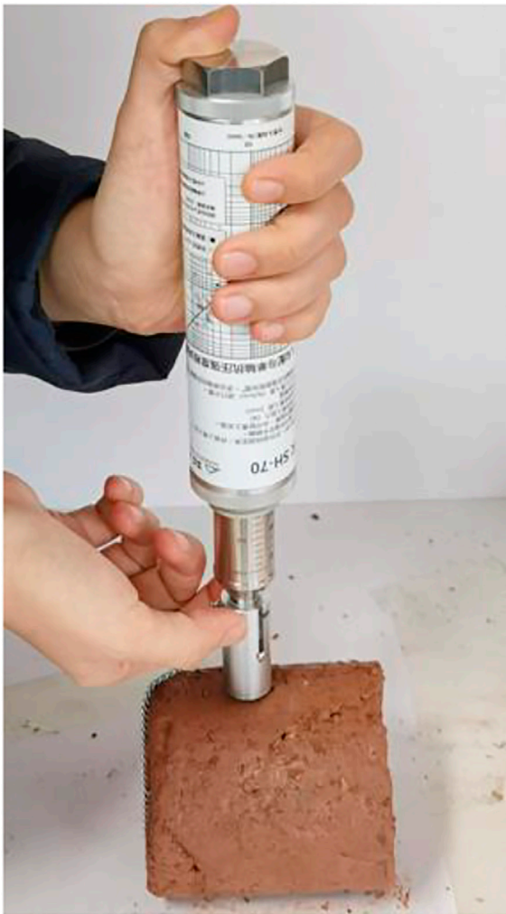
FIGURE 9 Needle penetration test on a mudstone core.
