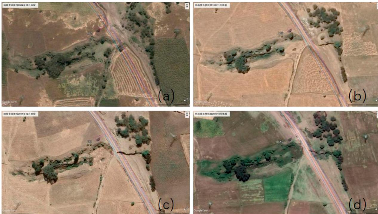
**FIGURE 7** Ground fissure development of the Arsi Negele connecting line: (A) remote sensing images, October 2004; (B) satellite remote sensing images, November; (C) remote sensing images, December 2017; and (D) remote sensing images, October.
