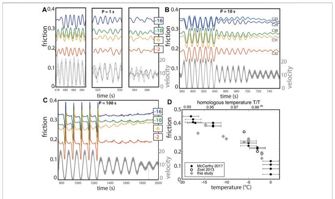
**FIGURE 3** | Frictional response to periodic load point velocity (gray) as a function of temperature between -16.4°C and -2°C, from samples C29 - C33 at, respectively, at **(A)** 1 s periods; **(B)** 10 s periods; and **(C)** 100 s periods. **(D)** Temperature directly affects the average friction, consistent with steady-state friction coefficients from previous studies (Zoet et al., 2013; McCarthy et al., 2017).
