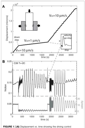
program. **(B)** Driving velocity in gray and measured friction (black) for a single run (C39) of ice sliding on rock in double direct shear (upper inset) at  $-2^{\circ}$ C.
