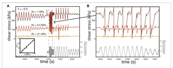
**FIGURE 6 | (A)** Shear stress response to periodic velocity as a function of normal stress, at T = -5°C. Data at 0.1 MPa is sample C34. Data at 0.5 and 1.0 MPa are from sample C41a and C41b, respectively. A plot of shear stress vs. normal stress (inset) demonstrates Coulomb behavior with no cohesion. **(B)** A magnification of the 10 s period data shows that at increasing normal stress, stick-slips and period doubling are observed.
