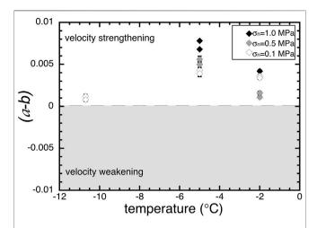
**FIGURE 8** | Rate dependence of friction, a-b, vs. temperature, from experiments C34-44 each measured from a velocity step from 1  $\mu$ m/s to 10  $\mu$ m/s using the GUI described in Skarbek and Savage, 2019. Where error bars cannot be seen, they are smaller than the symbol size. Analysis of velocity steps indicates only velocity strengthening behavior over this temperature/velocity range.
