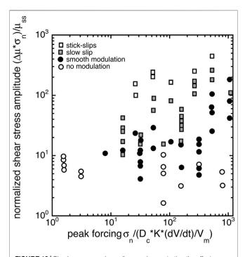
**FIGURE 10** | Simple response phase diagram demonstrating the effect of forcing rate on the frictional response style and amplitude (normalized delta friction multiplied by normal stress).
