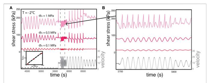
**FIGURE 5 | (A)** Shear stress response to periodic velocity as a function of normal stress, at T = -2°C. Data at 1.0 MPa is sample C32. Data at 0.5 and 1.0 MPa are from sample C44a and C44b, respectively. A plot of shear stress vs. normal stress (inset) demonstrates Coulomb behavior with no cohesion. **(B)** A magnification of the 10 s period data shows that at increasing normal stress, stick-slips are observed in the 1.0 MPa data.
