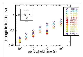
**FIGURE 4** | Frictional amplitude (inset) vs. period of forcing from this study (closed symbols) for those cycles that approach and reach zero velocity compared to change in friction and log hold time from previous slide-hold-slide experiments (open symbols) (McCarthy et al., 2017).
