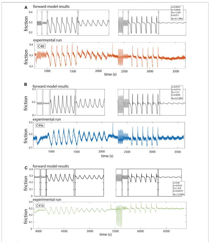
FIGURE 9 | Forward model results compared to three selected experimental runs. Values for models are those listed, which are determined from the velocity step analysis (Table 2) using the Slip form of state (A) at normal stress = 0.1 MPa; (B) at a mid-range of normal stress = 0.5 MPa; and (C) at highest normal stress = 1.0 MPa.
