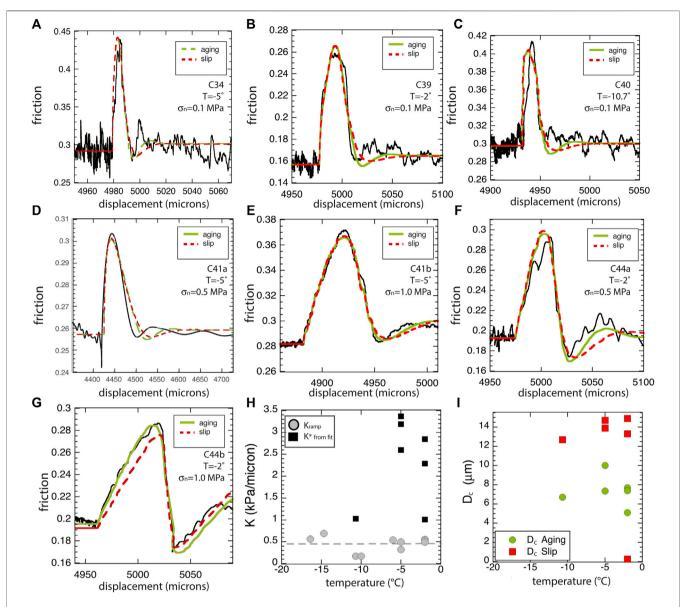
FIGURE 7 | (A-G) Velocity up steps from 1 to 10 microns/s from experiments C34-44 with curve fits (of both Aging and Slip laws) overlain. (H) fitted values of K from velocity steps and from the loading ramp as a function of temperature (at 0.1 MPa normal stress) and (I) D<sub>C</sub> (from Aging and Slip fits) as a function of temperature.
